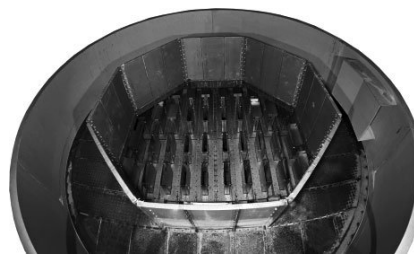
Figure 11. Flashing gallery for a packed mass transfer tower.
