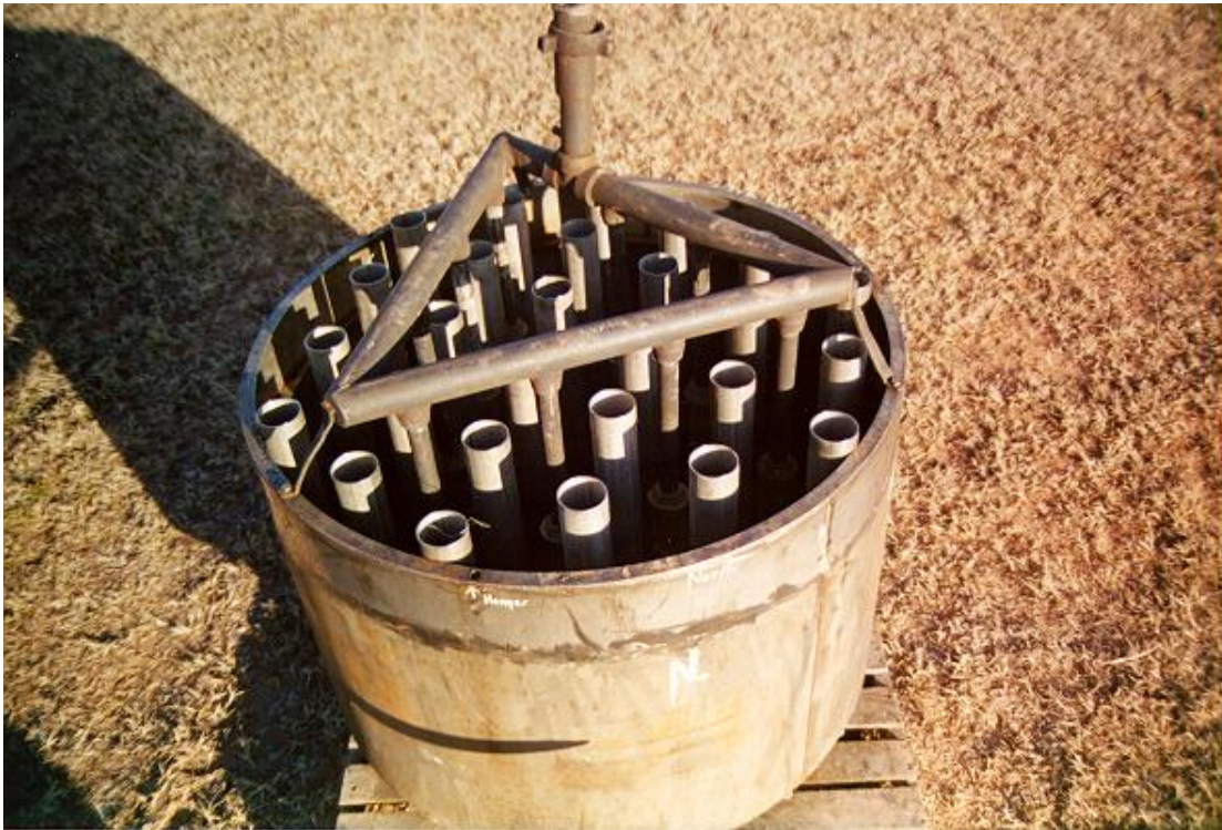
Figure 3. F.R.I. Tubed Drip Pan Distributor
