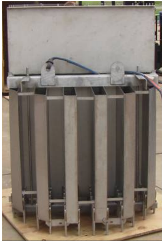
Figure 2. Raschig DT-S Liquid Distributor
