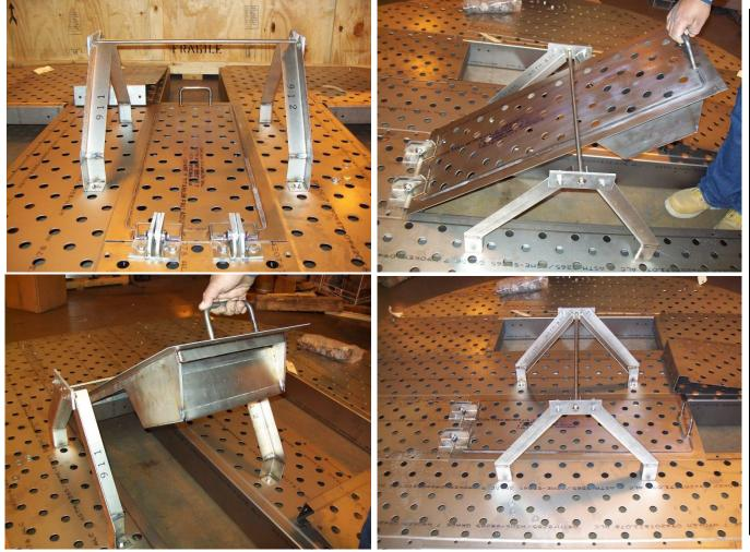
Raschig USA prepared the mechanical and process designs of the trays for this tower and then supervised the fabrication and assembly of the several trays required for the tower. The design included all aspects of the tray seen here – including the support arms in addition to the panel itself. Also please note manways included in the tray design on either side of the pressure relief hatch.
