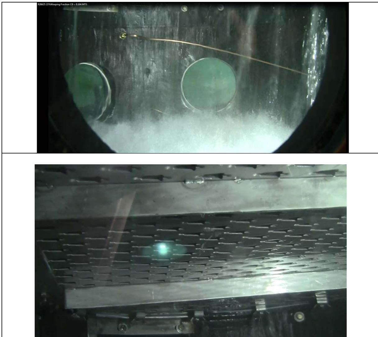
Fig. 4: Videotaped tray support ring leakage; top: column wall view between tray 3 and 4; bottom: view to tray 4 from below
