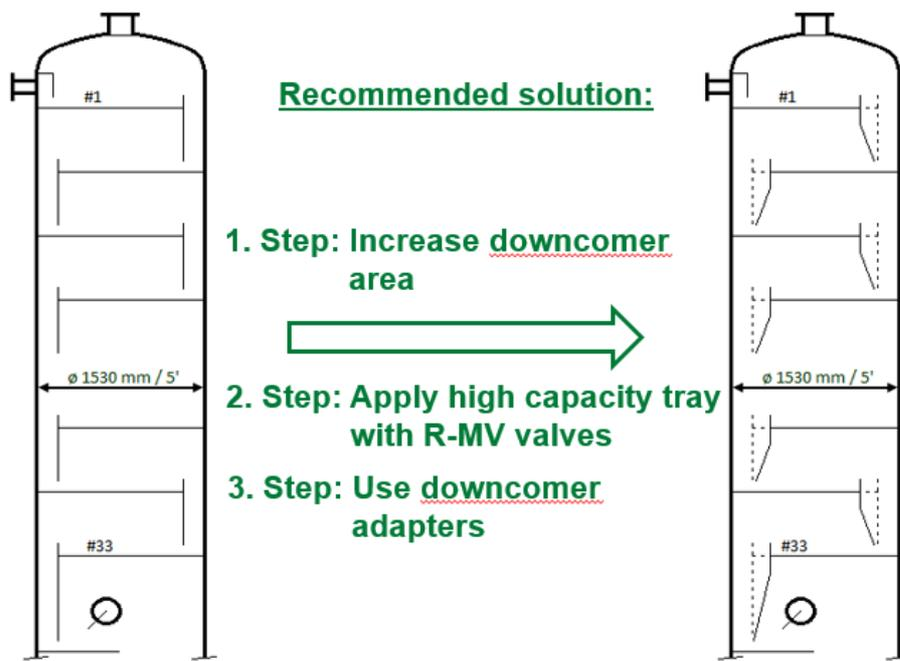
Fig. 11: Revamp of a distillation column from movable V1 valves to high capacity Raschig Mini Fixed Valves
