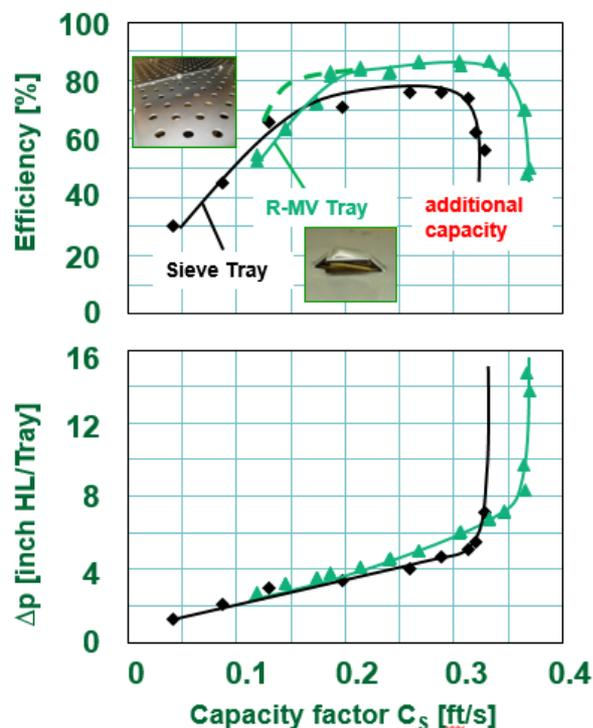
Fig. 9 Efficiency, pressure drop and capacity over column cross section area related  $C_s$ -factor of Raschig Mini Fixed Valves and sieve trays tested at FRI with cyclohexene/n-heptane at 1.62 bar (24 psia)
