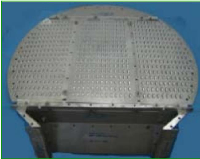
Fig 12: Tray deck layout applied for revamp project with Raschig Mini Fixed Valves and downcomer adapters
