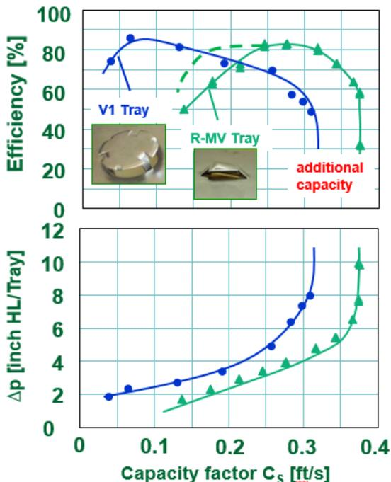
Fig. 8: Efficiency, pressure drop and capacity over column cross section area related  $C_s$ -factor of Raschig Mini Fixed Valves and movable V1 valves tested at FRI with cyclohexene/n-heptane at 0.31 bar (4.5 psia)
