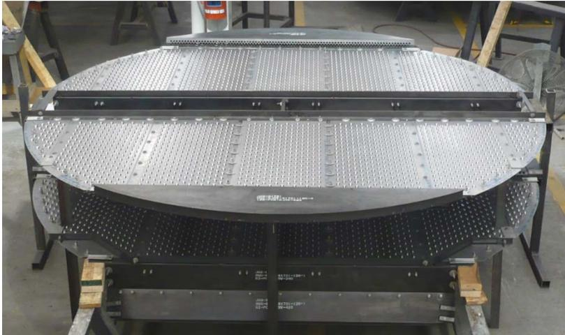
Fig 15: Tray deck layout applied for a grass root butane splitter project with Raschig Mini Fixed Valves and NYE inserts
