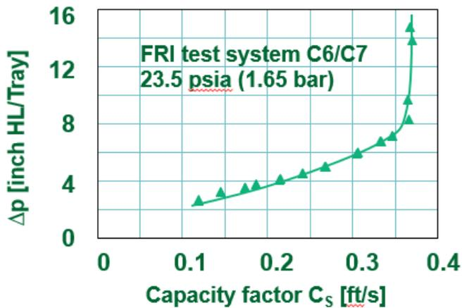
Fig. 5: Pressure drop and capacity over column cross section area related  $C_s$ -factor of Raschig Mini Fixed Valves tested at FRI with cyclohexene/n-heptane at 1.62 bar (24 psia)
