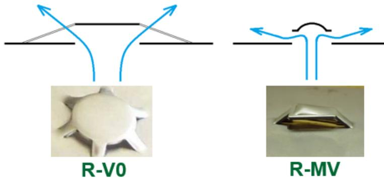
Fig. 2: Gas flow stream via a standard round fixed R-V0 valve and a high capacity R-MV Mini Fixed Valve by Raschig
