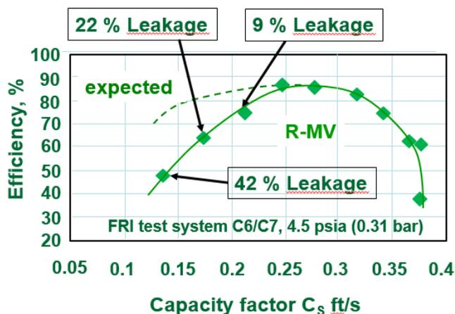
Fig. 6: Tray efficiency, capacity and tray support ring leaking fraction over column cross section area related  $C_s$ -factor of Raschig Mini Fixed Valves tested at FRI with cyclohexene/n-heptane at 0.31 bar (4.5 psia)
