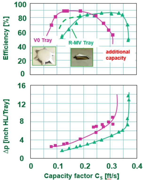
Fig. 10 Efficiency, pressure drop and capacity over column cross section area related  $C_s$ -factor of Raschig Mini Fixed Valves and fixed V0 valves tested at FRI with cyclohexene/n-heptane at 1.62 bar (24 psia)
