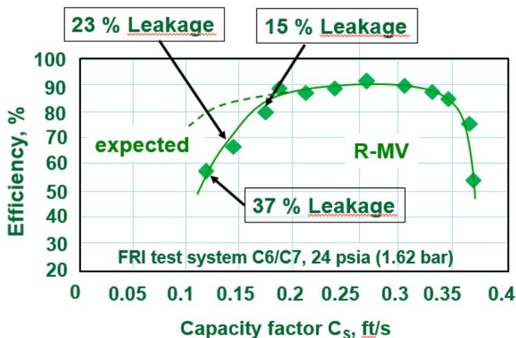
Fig. 3: Tray efficiency, capacity and tray support ring leaking fraction over column cross section area related  $C_s$ -factor of Raschig Mini Fixed Valves tested at FRI with cyclohexene/n-heptane at 1.62 bar (24 psia)
