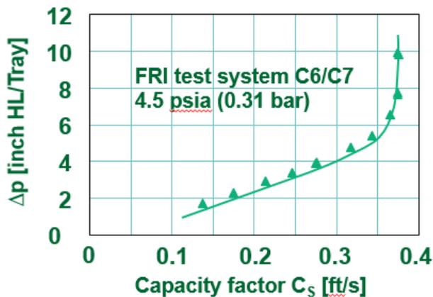
Fig. 7: Pressure drop and capacity over column cross section area related  $C_s$ -factor of Raschig Mini Fixed Valves tested at FRI with cyclohexene/n-heptane at 0.31 bar (4.5 psia)
