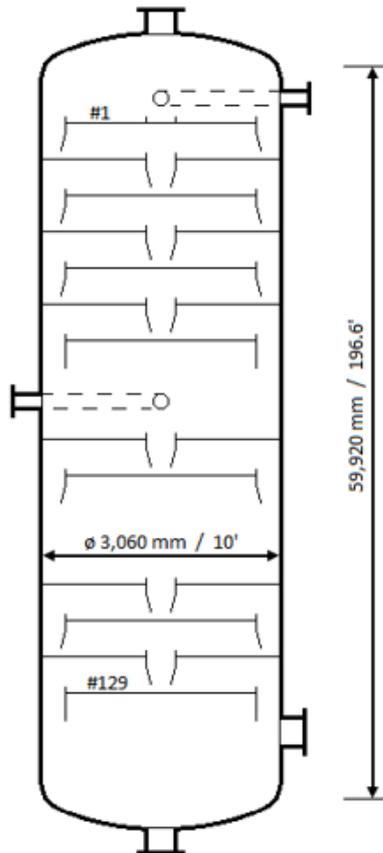
Fig. 13: Grass root design of a Butane Splitter with Raschig's to high capacity Mini Fixed Valves
